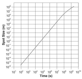
Fig. 5 Plot of DE-STAR spot size (reflector size required) with respect to time for the 100 kg craft case. This assumes the reflector is illuminated fully the entire time.
