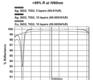
Fig. 9 Graph of the percent reflectance for a practical thin film roll to roll reflector design. The green line of 1,060 nm corresponds to DE-STAR's laser wavelength. (Source: figure and data from Surface Optics - private communications (2013)). Reflectivities in excess of 99.995% are achievable now on thin film plastics and with further refinements 99.999% looks feasible.
