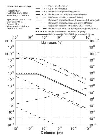
Fig. 10 Communications parameters between a DE-STAR 4 and a small robotic spacecraft vs. distance to spacecraft. The spacecraft is assumed to have a 10 watt burst mode (hibernates most of the time) IR transmitter and uses a 30 m reflector as both the drive and the transmit/receive reflector. Both uplink (DE-STAR to spacecraft) and downlink (spacecraft to DE-STAR) are shown.
