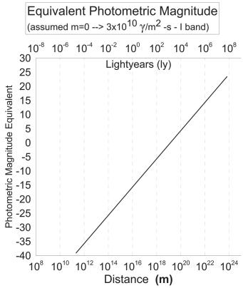
Fig. 12 Photometric (broad band equivalent) magnitude vs distance for a DE-STAR 4 out to 1 Gly. The I band equivalent photometric magnitude at 1 Gly form a DE-STAR 4 is approximate m=30 or roughly the limit of the HST.
