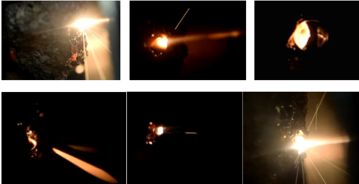
Figure 16. Various pictures of mass ejecta, sparks, plume, and bubbles due to laser ablation. These pictures show the environment at the sample while laser ablation is occurring. See online video.
